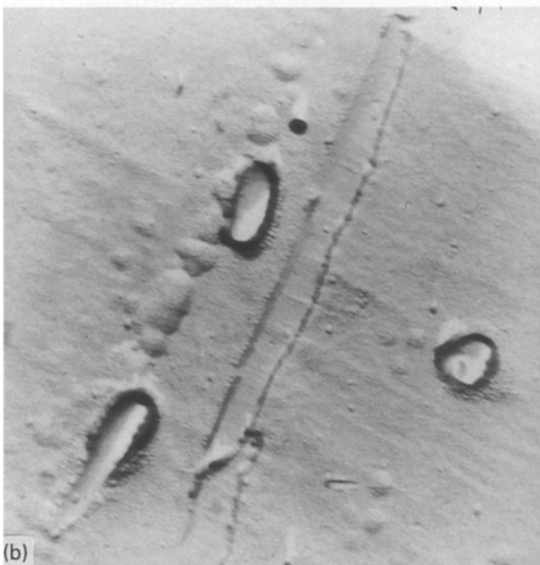
Figure 1 Transmission electron micrograph of an annealed specimen (920 °C for 3 h in argon) after fatigue tests at 95 MPa, R = -1 . (a) Dissolution of the ferrite–cementite interface resulting in the formation of microvoids. 6.26 \times 10^5 reversals; \times 11\,300 . (b) Fracture of inclusion and formation of intrusion-type defects at hydrogen blisters. 1.05 \times 10^6 reversals; \times 11\,300 . (c) Formation of subgrains and microcracks at subgrain boundaries after 1.05 \times 10^6 reversals; \times 8200 .
