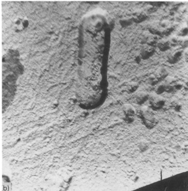
Figure 4 Transmission electron micrograph of an as-received specimen after 2000 reversals at 193 MPa, R = -1 . (a) Formation of hydrogen blisters and submicroscopic cracks near inclusions; \times 20\,500 . (b) Intersection of slip bands and hydrogen blisters; \times 20\,500 .
